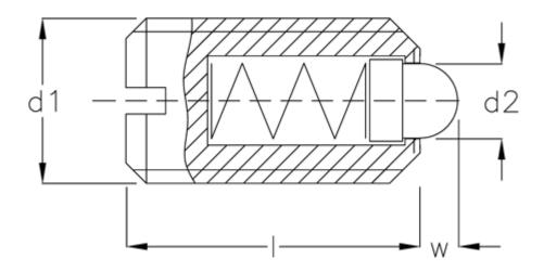
$\begin{array}{ll} \text{d1} & = \text{M24} \\ \text{d2} & = 13.0 \\ \text{Length I} & = 34 \\ \text{Spring pressure N bottom} = 155.0 \\ \text{Spring pressure N top} & = 72.0 \\ \text{W} & = 8.0 \\ \end{array}$
